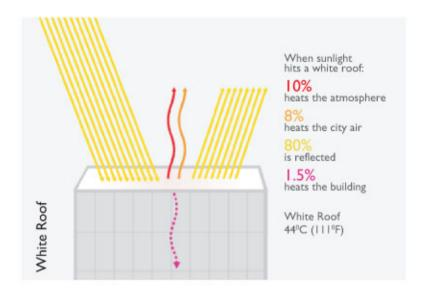
If all urban, flat roofs worldwide were whitened, the reduction in carbon emissions would be 24 Giga tones, or equivalent to taking 300 million cars off the road for 20 years. This is based on the fact that a 1,000-sq.ft (93 m2) white roof will offset 10 tons of CO<sub>2</sub> over its 20-year lifetime.
