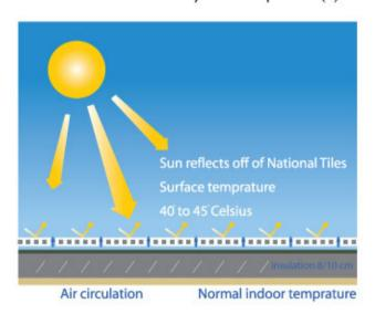
The results for both phases of the project, showed a 25.3% average reduction (8.6 kWh) in summer space cooling energy (34.1 kWh/day to 25.5 kWh/day) in the seven shops with a range of savings of 13 - 48%. The percentage savings varied with the temperature maintained in the shops; those maintaining the lowest interior temperatures saved theleast on a percentage basis.
